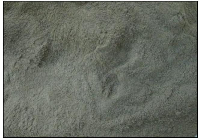
Fig 3 Ground Granulated Blast furnace Slag
